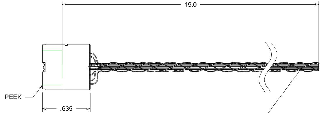
9EA 28 AWG. STRANDED WIRES WITH KAPTON INSULATION AND A PEEK BRAID.
