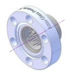
1-1/3 Mini 304ss / Fixed / CF Flange with clearance bolt holes 6x Ø.172 on Ø1.062 BC
